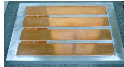
Direct contact VC epoxied to an aluminum heat sink
